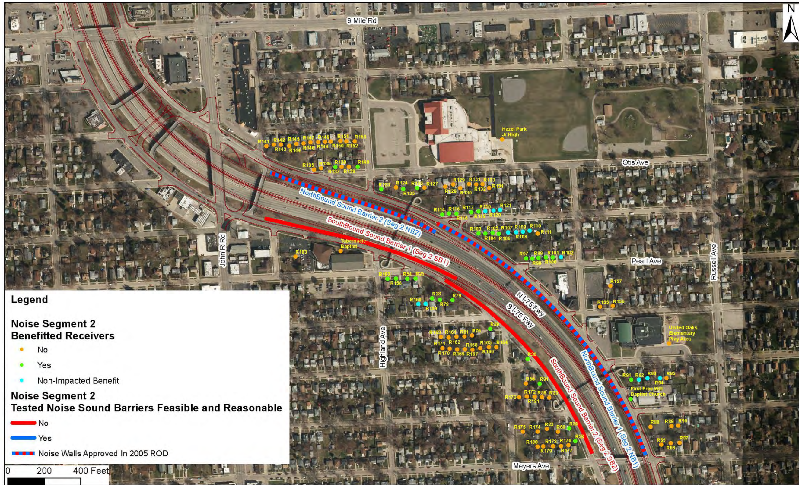
Figure 22 – Noise Segment 2 Sound Barrier Design Configuration for Benefitting Receivers Behind Northbound Barriers NB1 & NB2 and Southbound Barriers SB1 & SB2
